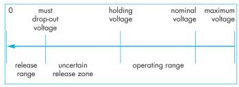
Non-operate voltage: The highest value of input voltage at which the relay will not operate (not specified in the catalogue).
