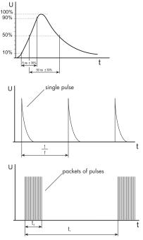
2. **Surge** (voltage pulses). These are single **1.2/50 \mus** pulses, with energy much higher than bursts since the duration is considerably longer - 1.2  $\mu$ s rise time (1.2  $\times$  10° seconds) and 50  $\mu$ s fall time.
